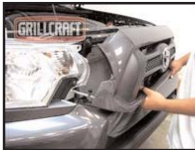
REMOVE GRILLE SHELL FROM VEHICLE.
