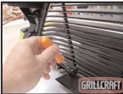
WHILE HOLDING GRILLE INSERT IN PLACE MARK MOUNTING BRACKET CENTER HOLE LOCATIONS.
