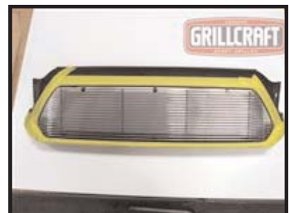
PLACE GRILLE INSERT INTO GRILLE SHELL.
