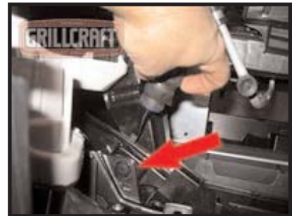
REMOVE PLASTIC CLIP LOCATED ON RIGHT & LEFT LOWER BACKSIDE OF THE GRILLE SHELL.
