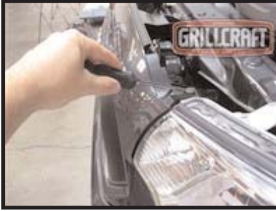
USING A SCREWDRIVER UNCLIP THE PUSH CLIPS ALONG THE TOP OF THE GRILLE SHELL.
