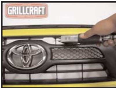
PROTECT THE GRILLE SHELL FROM GETTING SCRATCHED USING MASKING TAPE. START BY CUTTING THE CENTER SECTION OF THE GRILLE SHELL OUT FIRST
