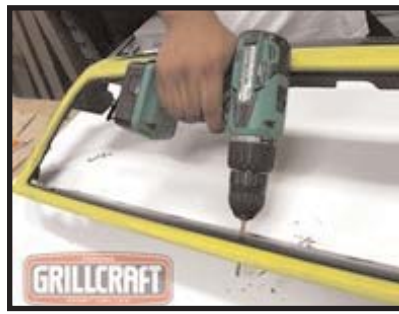
DRILL HOLES FOR THE GRILLE INSERT MOUNTING SCREWS.
