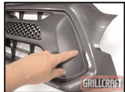
THE FACTORY GRILLE CENTER NEEDS TO BE CUT OUT. PLEASE REVIEW CUTTING INSTRUCTIONS BEFORE CUTTING GRILLE CENTER.
