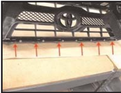
IN ORDER TO REMOVE GRILLE SHELL YOU MUST UNCLIP THE SIX PLASTIC TABS ALONG THE BOTTOM OF THE GRILLE SHELL. PULL FORWARD ON THE GRILLE SHELL WHILE UNCLIPPING TAB FROM THE BACK SIDE ONE AT A TIME.
