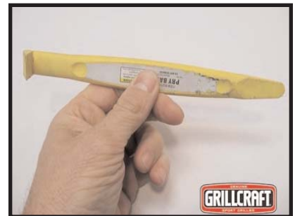
We recommend using a "Nylon Pry Bar" in order to remove grille shell clips. Nylon Pry Bar are available at Harbor Freight Tools. Item# 95214 www.harborfreight.com
