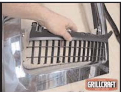
Removing end sections of the grille shell.
