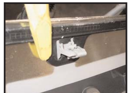
A close up of the grille shell clip.
