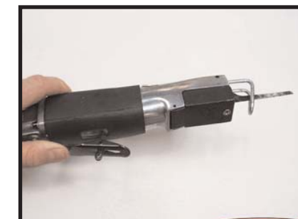
We are going to use a air saw for the cutting of the grille shell center.
