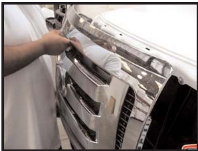
Now remove grille shell from vehicle.
