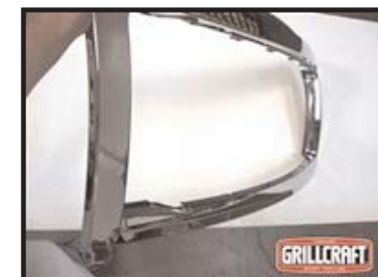
Another view of the grille shell ready for the grille center.Using a small disc grinder works well to clean up cut lines.
