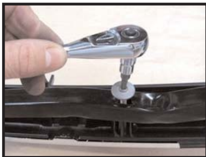
Remove grille shell reinforcement bar . The screws are located on the backside of the grille shell.
