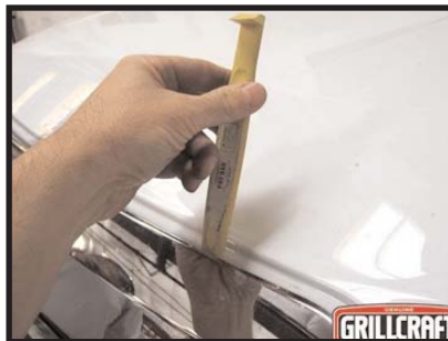
Place plastic pry bar under grille shell in order to release grille shell clip.
