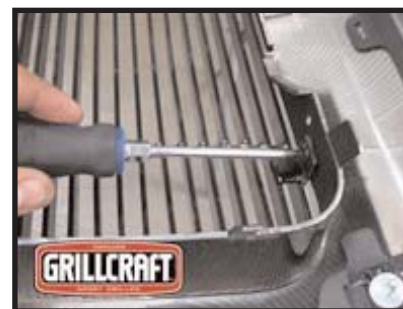
Another view of the top mounting screws. Next reinstall grille shell reinforcement removed in step #8.
