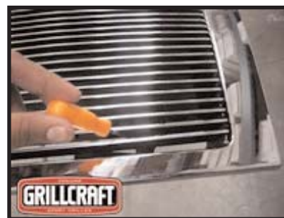
While holding grille into place mark mounting tab center hole location onto grille shell.
