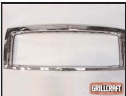
The factory grille shell with center section completely removed.
