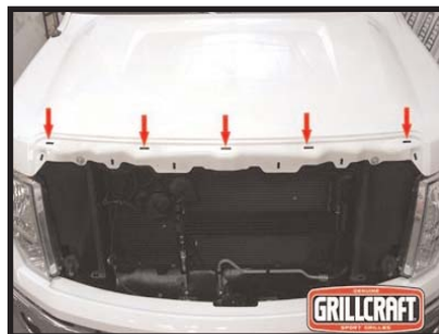
Note: locations of the grille shell clips.
